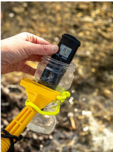
Conductivity meters are used to measure the amount of salt in aquatic environments.
